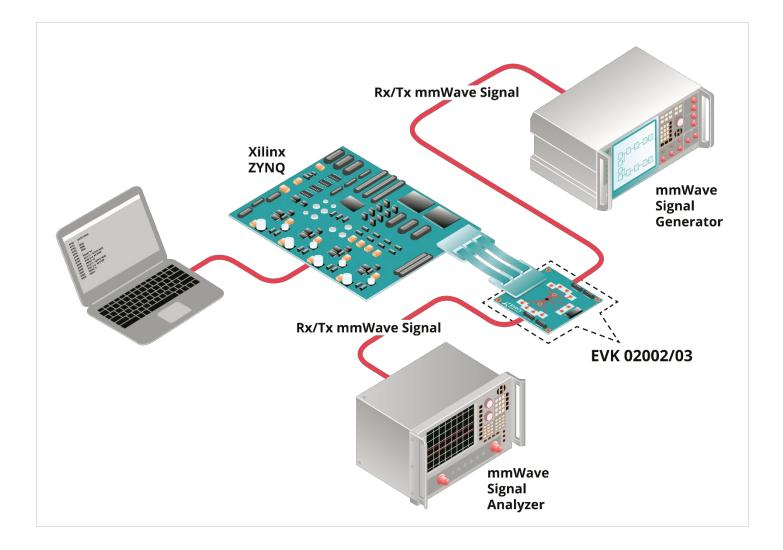
The evaluation board containing AFE VM 2Q 275/295 is controlled using a Xilinx Zynq board due to the high speed LVDS interface requirement. Software for easy configuration and display of results is included in the EVK kit.
