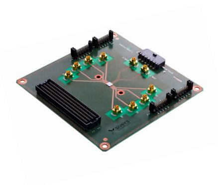
The Evaluation Kits (EVKs) are designed to help you validate the RF part of your 5G mmWave system. They help you Plug and Play with a minimum of configuration activities and are easily controlled through standardized interfaces. Configuration support and user guidelines are included.
